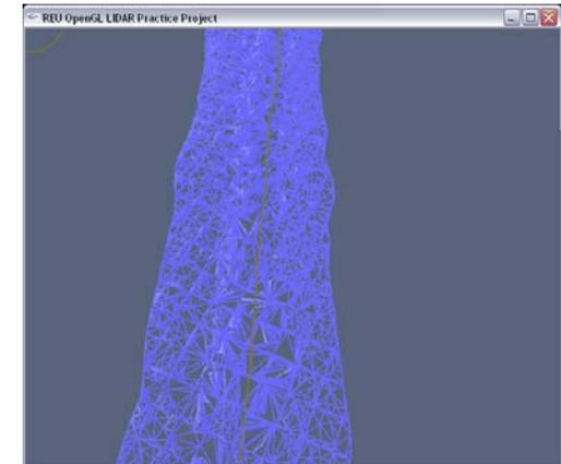
Figure 4: Triangulation of LIDAR data
