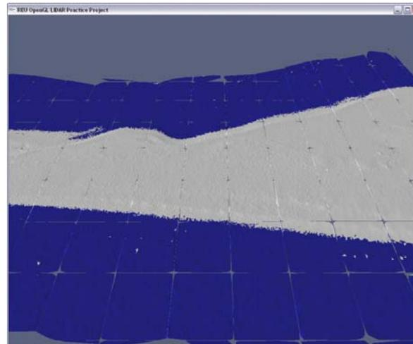
Figure 3: 3D processed LIDAR data with water and land shaded different colors
